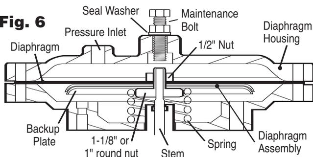
6. Using a back-up wrench on the plug, remove the stem nut on the shaft under the plug. Once the stem nut is broken loose, the 9/16" head maintenance bolt and top assembly will keep the stem from turning. The plug turns freely on the stem once loose. The plug and seat can now be removed. All soft seals should be replaced. Refer to kit part numbers under service parts on page 4.
