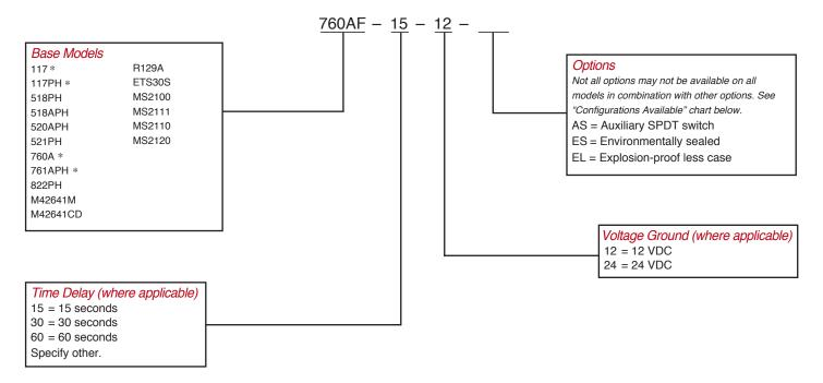
\* Add the letter "F" to the base model to indicate an inline fuse instead of a base mounted fuse. Example: 760AF, 761APHF, 117F.
